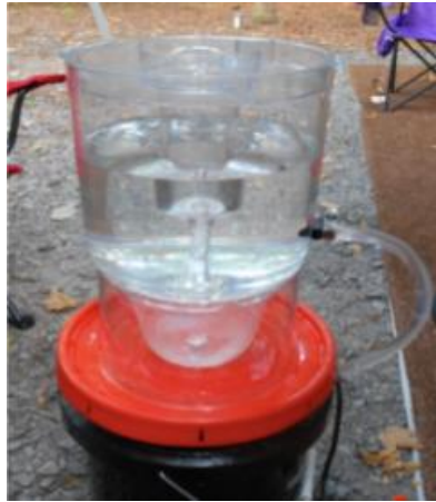
Figure 3: Pump whirlpool system. Intake bottom, outputs top right [4].
